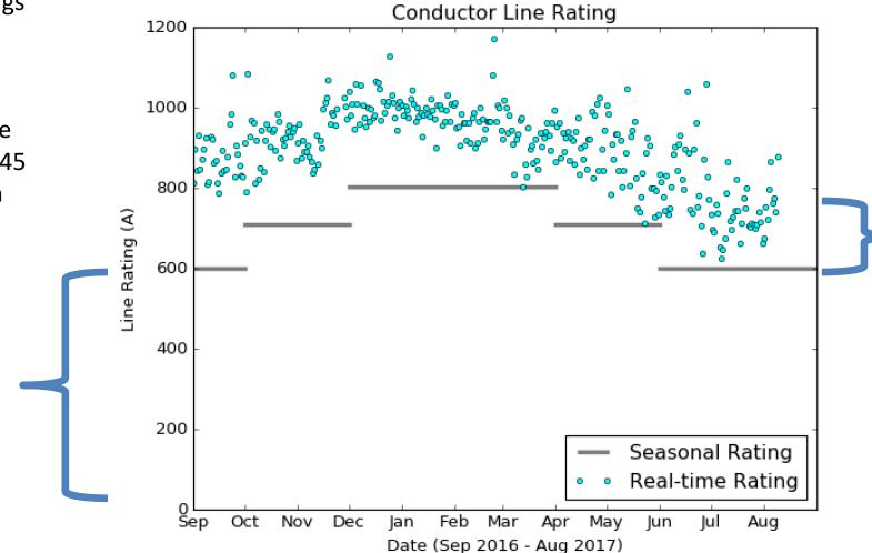
There is extra capacity between the seasonal rating and the real time rating. Dynamic line ratings could allow this capacity to be used.
