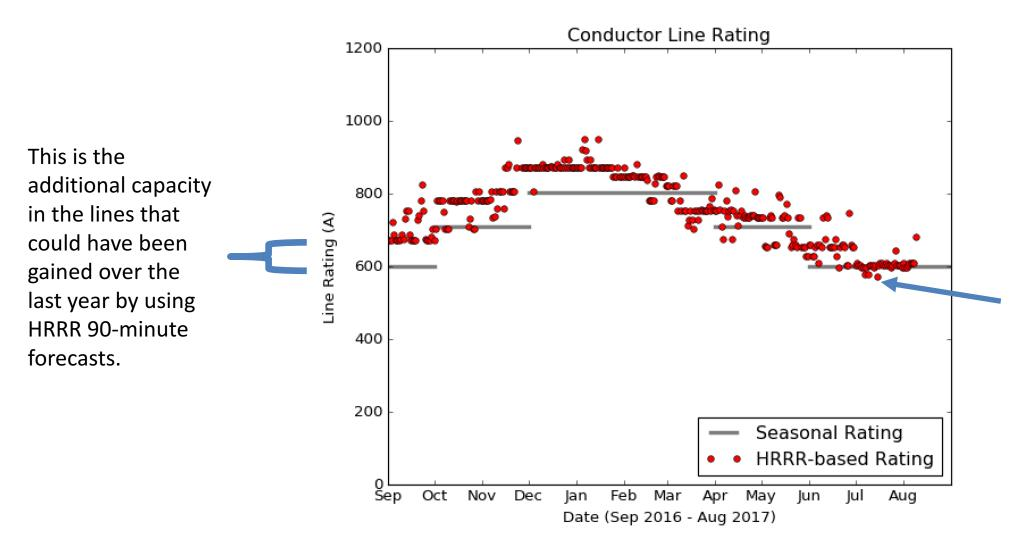
There are some times, particularly during the spring and summer, where using the HRRR forecast would have led to a lower line rating, which includes the safety factor.
